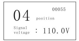
04 -- tap position signal; 00055—operation counter; signal voltage-110.0V
